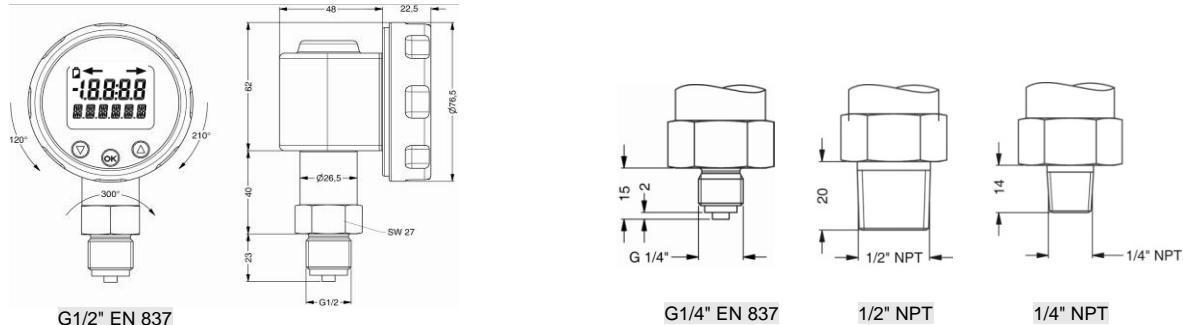
⇒ for nominal pressure  $P_N > 60$  bar increases the length of devices by 9 mm!
