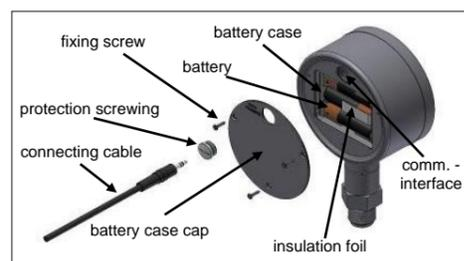
Fig. 3 Battery case and communication interface
